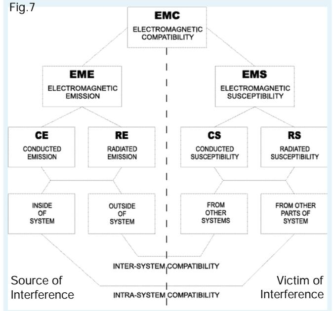
Fig.7 shows the EMC concept. Methods for evaluating the test results, emission limits, and immunity levels are quoted on the European Standards EN ... issued by CENELEC. Restriction on free circulation at EC level will be applied if equipment is found not to be in compliance.
