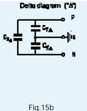
Considering the star-delta transformation, equivalent filtering from a star circuit compared with a delta network is obtained when  $C_x \gg C_y$  (i.e. in most cases) by using a value of  $C_2$  in Fig.15a, which is approximately twice  $C_y$  in Fig.15b. In any case the following transformation formulas are valid:
