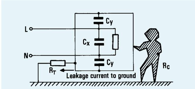
Fig.12 Besides the leakage current due to the filter, that associated with the equipment must be taken into account. All these currents are cumulative at the protective earth conductor. This total current cannot exceed the limit value, set by the safety specifications of the various national regulatory bodies and this depends on the type of equipment under consideration.
